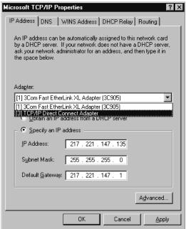
Figure 5-20. Select TCP/IP Direct Connect
